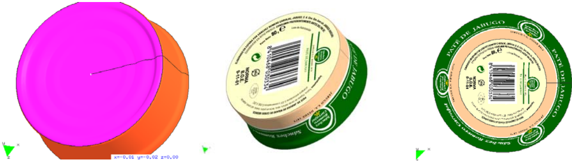
Fig. 4: Can stamping simulation made by Quantech ATZ for Metalpack SA: after deforming the sheet mesh to the final can state, the decorative labels are applied to the mesh and then its original flat shape is restored to get the deformed images, ready for the press ( courtesy of Quantech ATZ, Metalpack SA).
